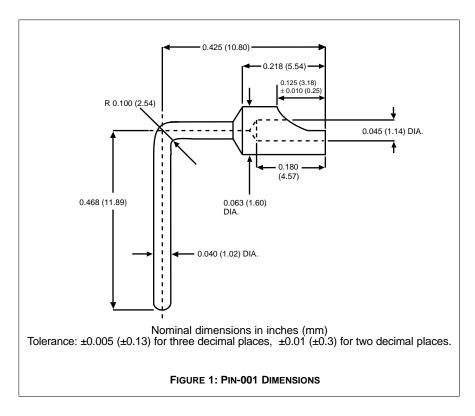
To prevent unwanted solder reflow, Interpoint suggests the use of SN 96 (high-temp solder) to connect the PIN to the converter terminal and SN 62 to connect the PIN to the board. The soldering restrictions referenced on the data sheets of the listed Interpoint products are 300°C for a maximum of 10 seconds per terminal.
